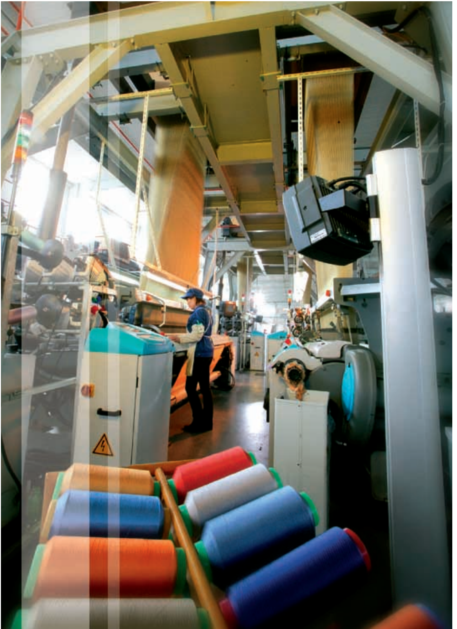
Sophisticated advanced computerised European Jacquard Looms in our new weaving plant
